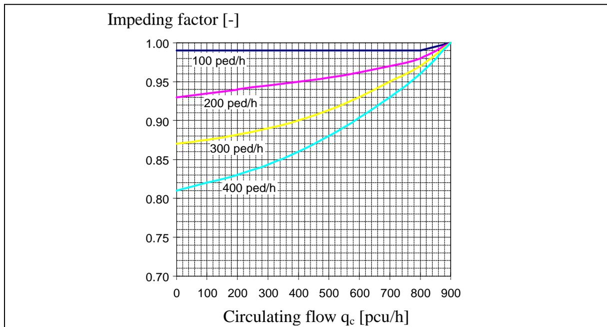
**Figure 12:** Impeding factors due to pedestrians at roundabouts with one circular lane
