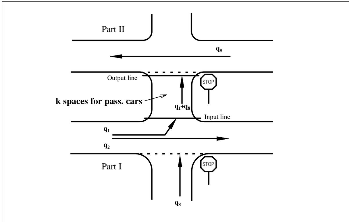
**Figure 1:** Minor street through traffic (movement 8) crossing the major street in 2 phases. The theory discussed here is also available if the major street provides more or less than 2 lanes per direction.
