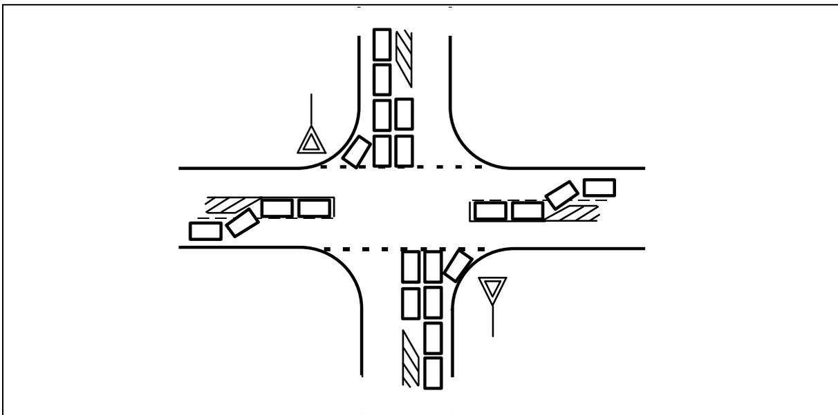
**Figure 3:** Possible queues at the approaches to an unsignalised intersection
