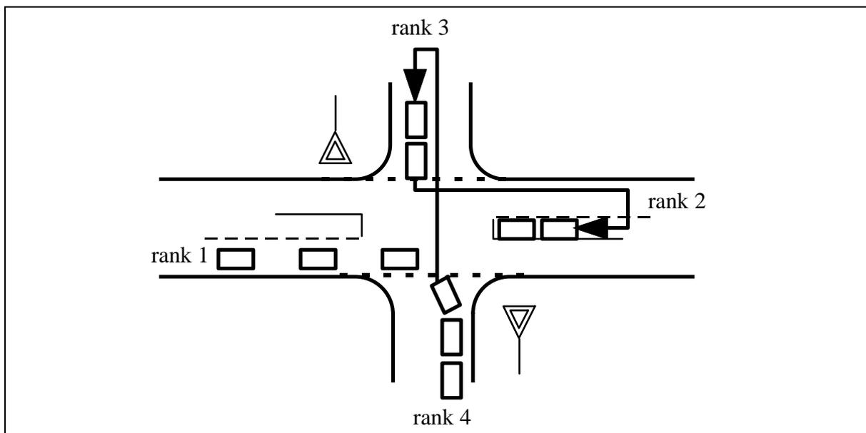
**Figure 4:** Queues in streams of different ranks and their sequence of operation
