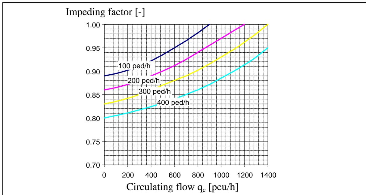
**Figure 13:** Impeding factors due to pedestrians at roundabouts with two circular lanes
