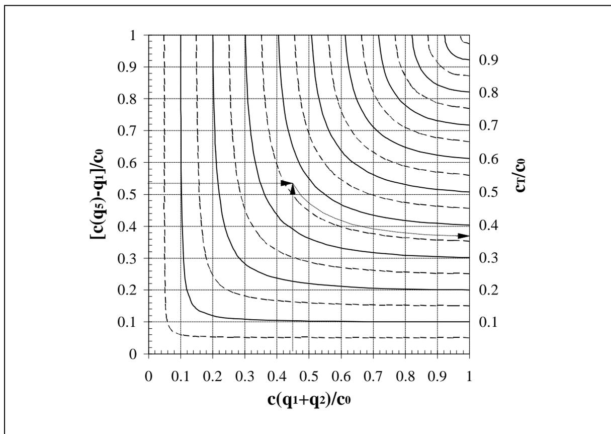
**Figure 2:** Capacities  $\hat{c}_T = c_T / c_0$  for movement 8 in relation to standardized values of capacities and of  $q_1$  (for  $k=2$ )
